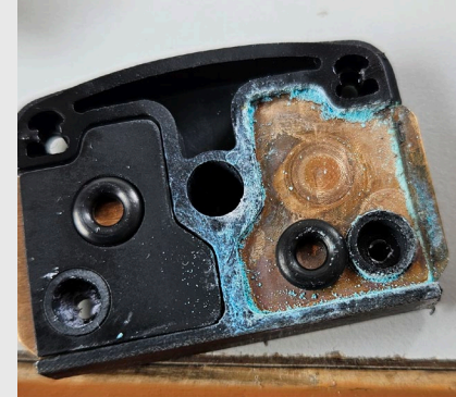
Corrosion on charging electrode
